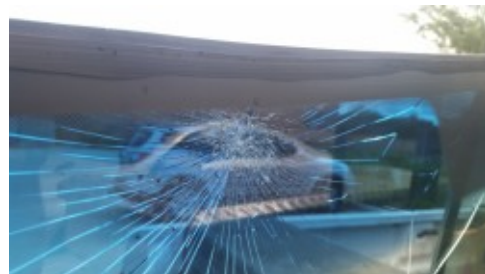
Golf Ball Damaged Windscreen Already Removed
